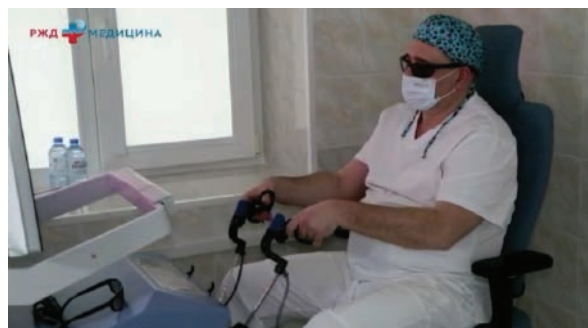
Figure 2. Cockpit with the technology of intelligent guidance of the video camera «Eye-Sensing Control» and tactile feedback
